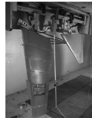
Fig. 9 Half-span F-111 (Wright-Patterson Flight Dynamics Laboratory design) wing-tail flutter model employed in damaged-wing study [34].
